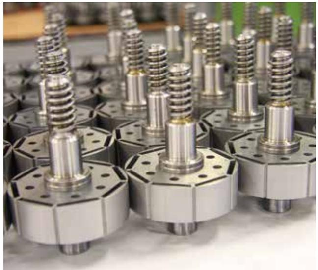
A digital brushless motor with permanent magnetic field, digital electronics for the complete management of the automation system control. Designed for super intensive use with the added benefit of a super low power consumption.
